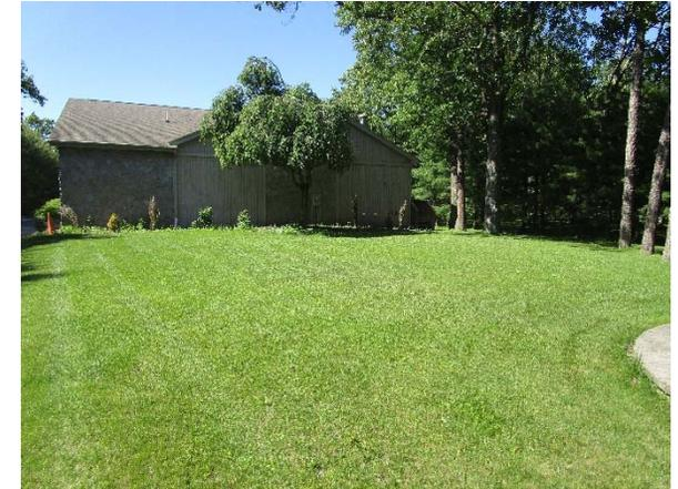
A rain garden can be installed in the turfgrass in front of the church when entering from the main road to capture, treat, and infiltrate stormwater runoff from the roof. A preliminary soil assessment suggests that the soils have suitable drainage characteristics for green infrastructure.
