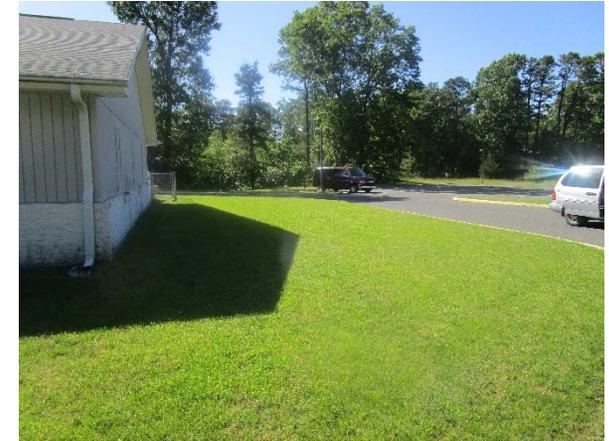
A rain garden can be installed in the turfgrass in front of the main entrance to capture, treat, and infiltrate stormwater runoff from the roof and pavement. Another rain garden can be installed in the turfgrass in the back of the church near the parking lot to capture, treat, and infiltrate stormwater runoff from the roof. A preliminary soil assessment suggests that the soils have suitable drainage characteristics for green infrastructure.
