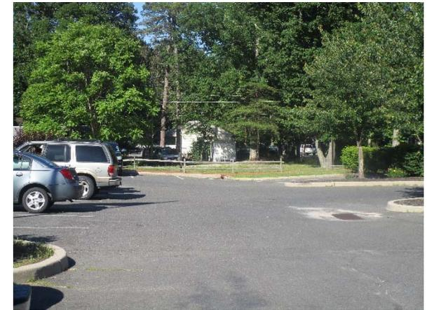
A rain garden can be installed in the turfgrass area west of the building to capture, treat, and infiltrate stormwater runoff from the roof. Parking spots on the east side of the lot closest to the entrance from the road can be converted into pervious pavement to allow stormwater flowing from the pavement to slowly infiltrate into the ground. A preliminary soil assessment suggests that the soils have suitable drainage characteristics for green infrastructure.
